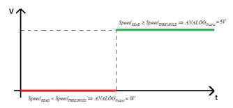
To activate this feature, the **Holding Register 46** must be set at value 2 and the required Speed Threshold value must be set into the **Holding Register 55**. The digital output of the driver changes its status (see above figure).
