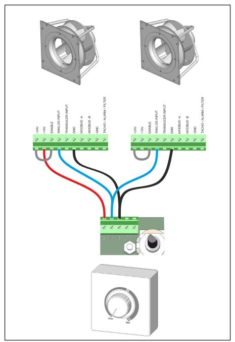
If an ext. 4-20mA device is used, it is necessary to add 0.1% precision resistances between the ANALOG INPUT and GND. The value of the resistance can range from:
