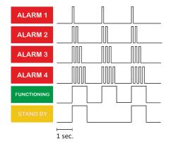
The system status can be displayed through the LED on the driver plate (see par. 9.6).
