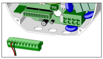
The voltage provided on the Enable input does not affect the four "Modbus - Temporary" modes, where the fan is intended to be completely controlled, including its starting and stopping, via its serial interface. This voltage is relevant in all the other operating modes: the modes relying on target values stored in fixed registers (Modbus – Fixed values) and the modes where an Analogue Input signal is used, plus the Master/ Slave mode.
