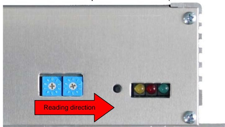
Figure 14: Alternatively Fan Controller Address Decimal Switches
