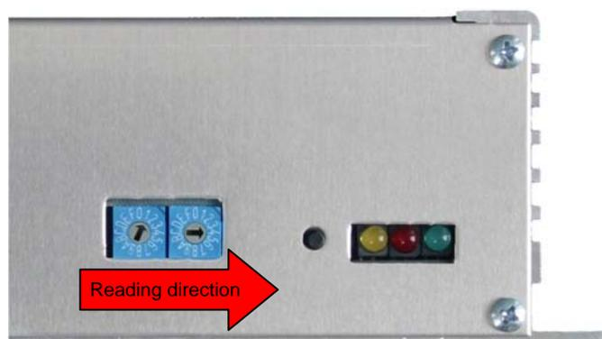
Figure 13: Fan Controller Address Switches
